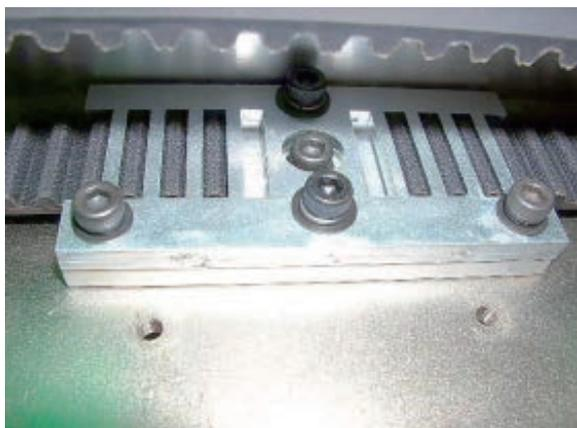
8. Referring to [3-7-1 Adjustment of X carriage belt tension], adjust tension of belt.
