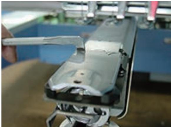
2. Adjust slant of fixed knife with [upper adjustment screw] and [lower adjustment screw] that fix fixed knife.
