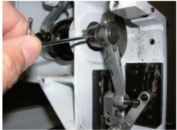
2. Remove pressure foot arm ass'y. (Fixing screw 2 pcs)
