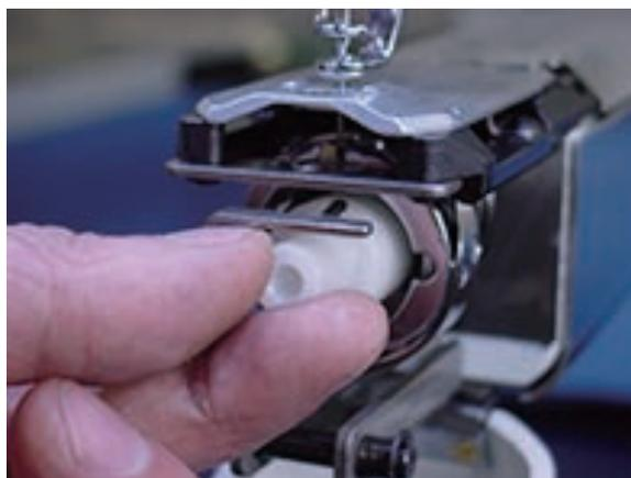
7. Adjust the needle bar height up and down till the needle tip touches to the gauge slightly.
