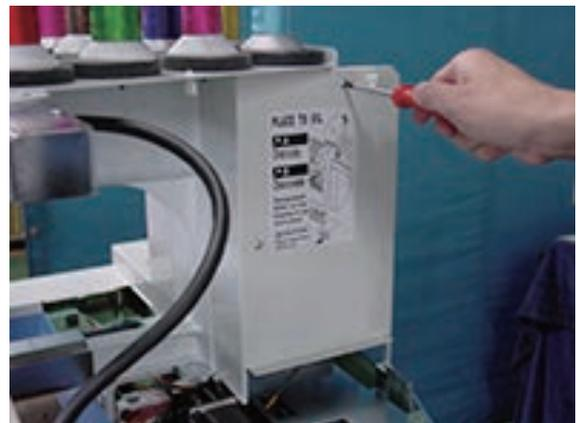
7. Remove the cover D. (Fixing screw 2 pcs)
