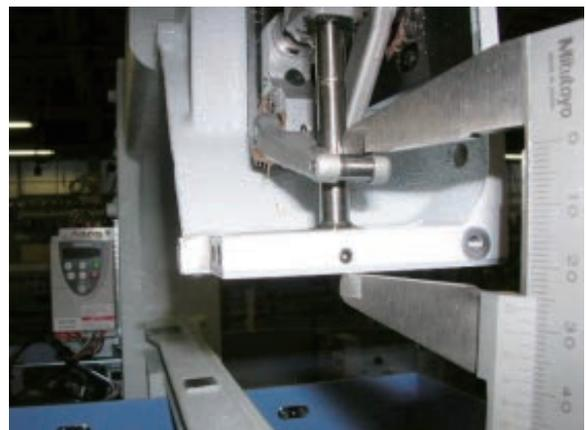
7. After check item 5 and 6 then tight screw completely for fix take-up lever cam.
