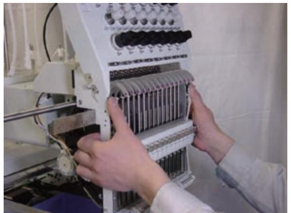
6. place a moving head on the thread guide.
