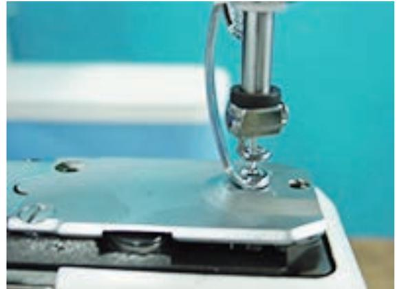
3. After adjustment, please be sure to check and adjust clearance between needle and shuttle hook.
