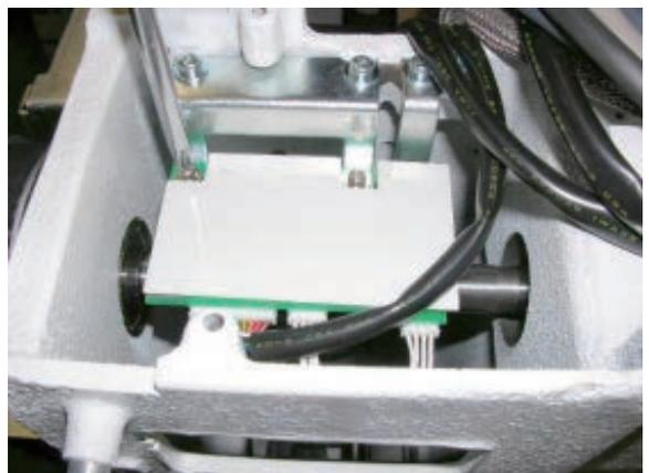
16. Remove detecting board bracket. (Fixing screw 2 pcs)
