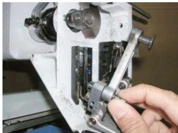
4. Loosen screw on rod. (Fixing screw 2 pcs)
