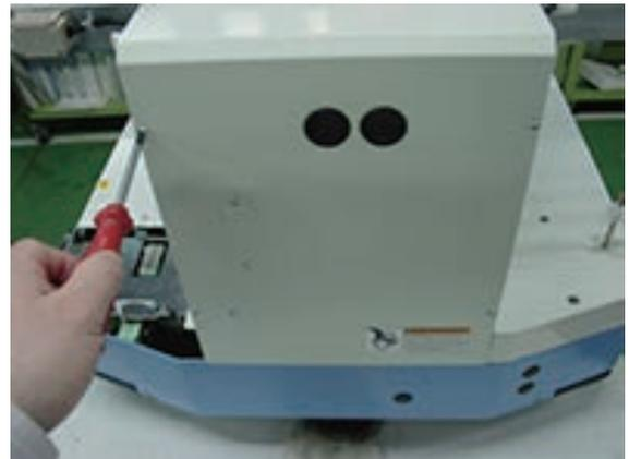
6. Remove the cover A. (Fixing screw 2 pcs)
