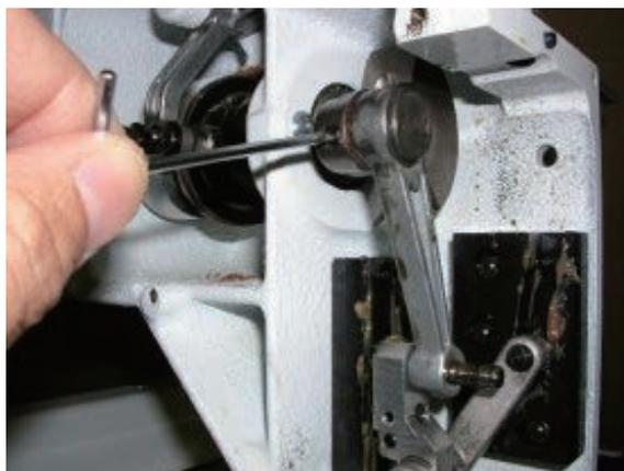
2. Remove pressure foot cam. (Fixing screw 3 pcs)
