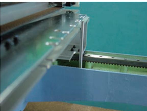
12. Touch X carriage body to pin gauges.
