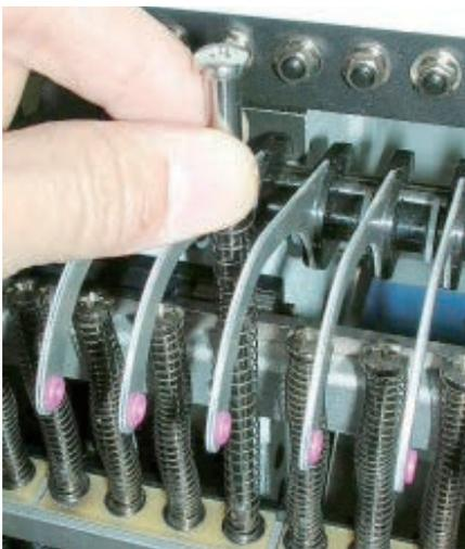
At this time, remove pressure foot spring (lower), pressure foot block, cushion and needle bar boss.
