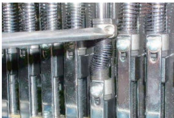
6. Put needle height gauge in rotary hook.
