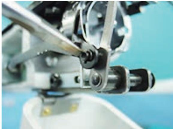
4. Remove Keeper ass'y. (Fixing screw 2 pcs)
