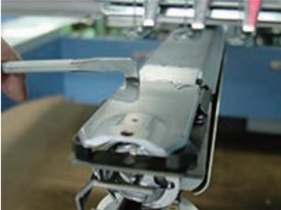
2. In case of you would like to replace rotary hook to new one, please remove retainer on bobbin case holder and loose three screws on rotary hook.
