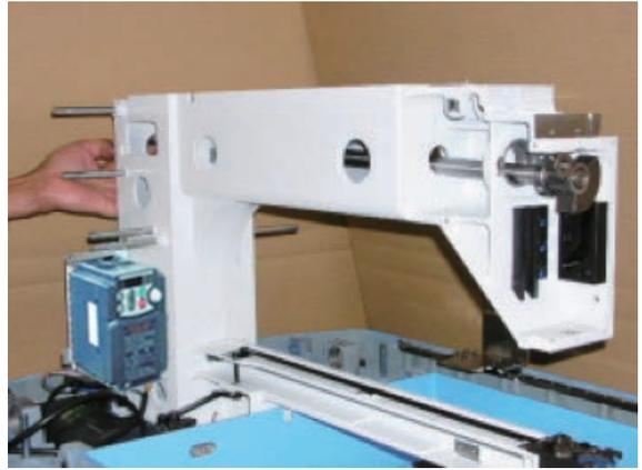
31. Please slide and off upper shaft collar, slit, Timing slit and take up lever cam from Clank ass'y
