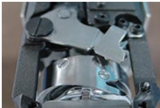
Loosen screw on link pin. (Fixing screw 1 pcs)
