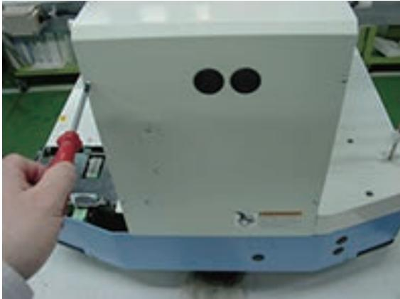
2. Loosen the screw on tension ass'y. (Fixing screw 2 pcs)
