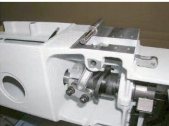
13. Loosen the screw on fasten collar with barrel cam.
