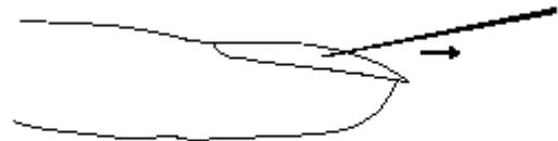
Please place needle on flat surface and check clearance (A) from side.
