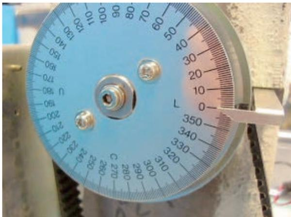
3. Turn detecting slit clockwise from pointer scale to set the position where LED4 goes out and tighten setscrews. (When detecting slit cover in L point sensor, LED4 goes out.)
