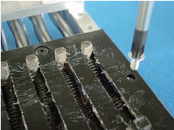
4. Fix positioning needle bar boss check plate.
