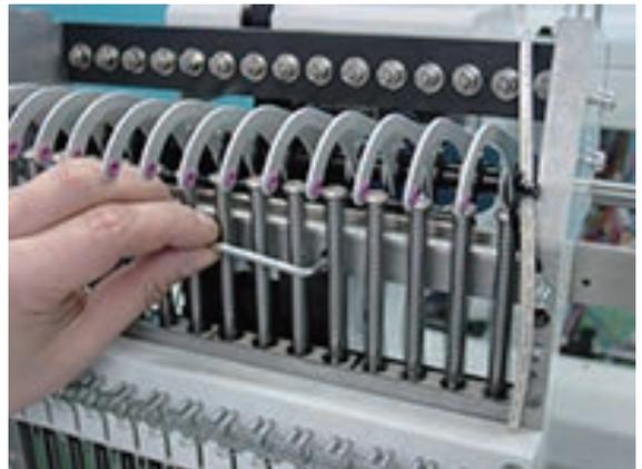
5. Remove it by holding moving head up.
