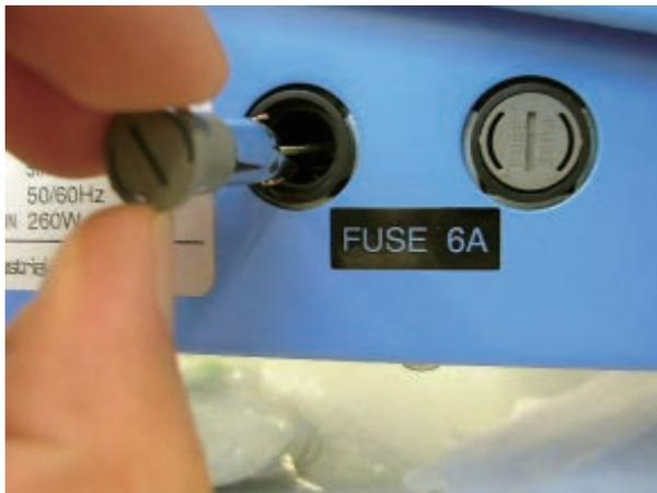
3. Remove fuse from fuse cap holder.
