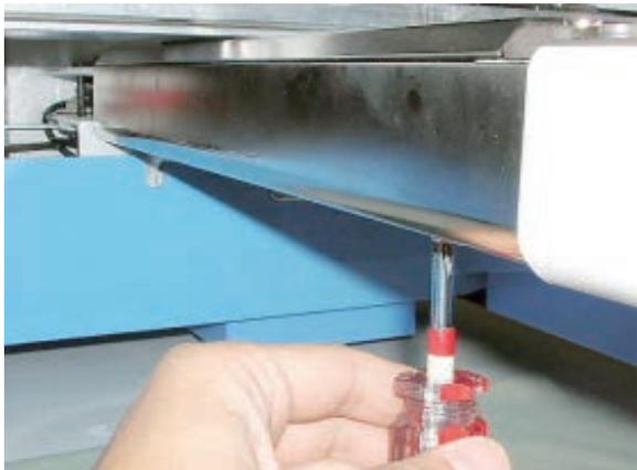
2. Remove connector for keeper solenoid.
