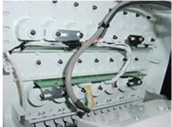
5. Slide TC8-7 circuit board for slit position to center of the sensor.
