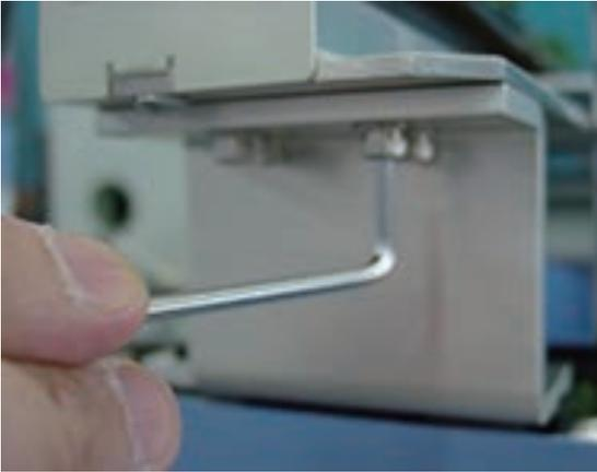
11. Insert positioning pin gauge 6mm.
