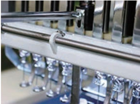
2. Loosen screw on needle bar boss.
