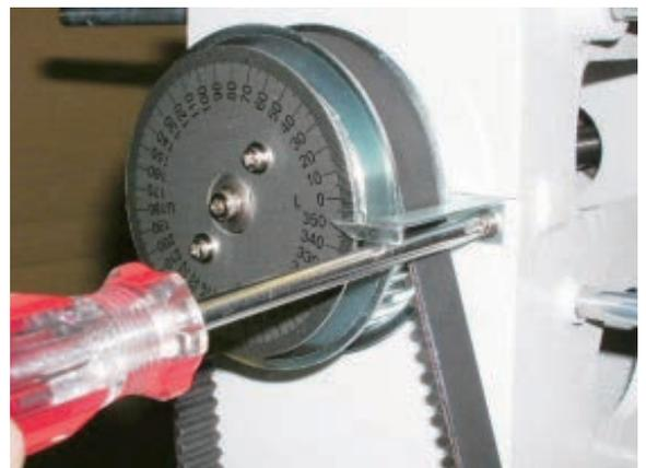
22. Check clearances between tension ass'y and tension block for 6.5mm to 7.0mm.
