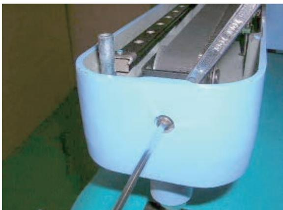
4. Remove belt holding plate. (Fixing screw 2 pcs)
