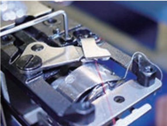
3. Adjust height of bobbin thread holder with adjusting screw.
