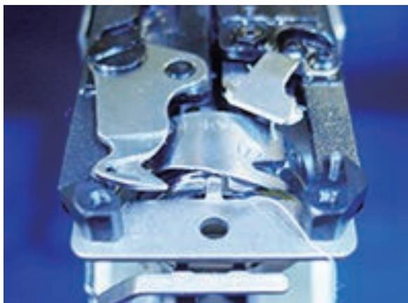
4. In this condition, Turn link pin till moving knife maximum opened point and fix link pin.
