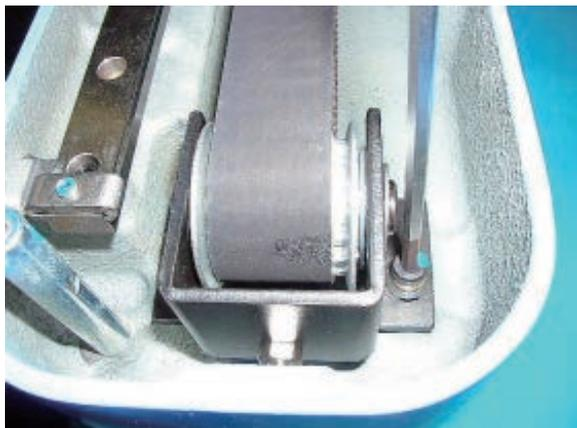
9. Check belt tension again then tighten lock nut.
