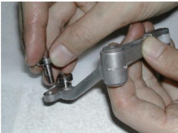
3. Insert bering positioning gauge [4.85mm] between bering and bering, and then tighten roller shaft ass'y.
