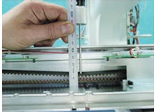
4. Push the belt by tension gauge at 1.5kg and measure distance between connecting plate and top of the belt. (0.5kg Wide X carriage)
