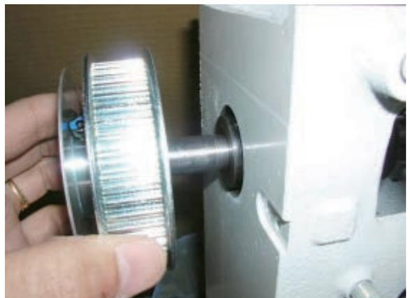
28. Slide clank ass'y in upper shaft to front side of machine.
