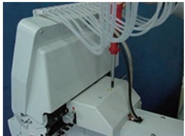
11. Remove the head left side cover. (Fixing screw 2 pcs)
