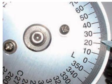
5. Adjust rotary hook timing.
