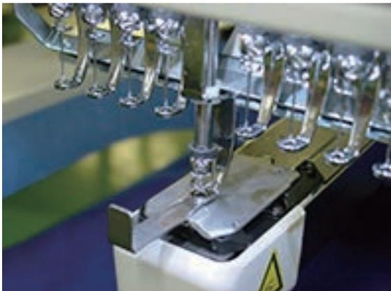
10. Tighten fixing screw for pressure foot.
