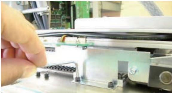
5. Remove belt holding plate. (Fixing screw 4 pcs)
