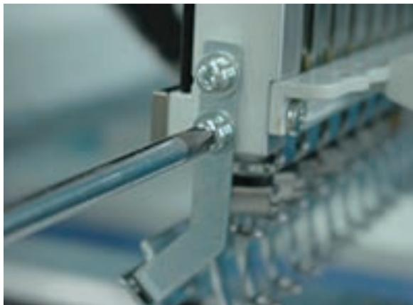
2. Remove holder (lower). (Fixing screw, nut 2 pcs)
