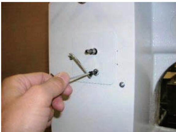
Remove the bobbin thread guide. (Fixing screw 2 pcs)
