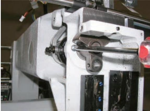
11. Remove take-up lever crank. (Fixing screw 1 pcs)
