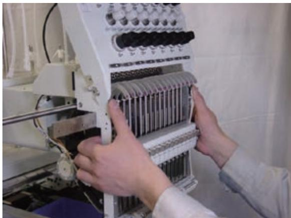
2. Loosen screw on take-up lever shaft. (Fixing screw 2 pcs)
