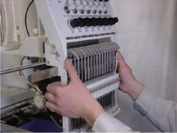
2. Exchange of needle bar boss check plate.
