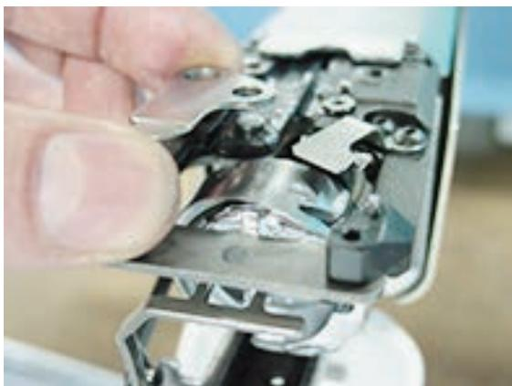
6. Fix moving knife with knife shaft and nut.
