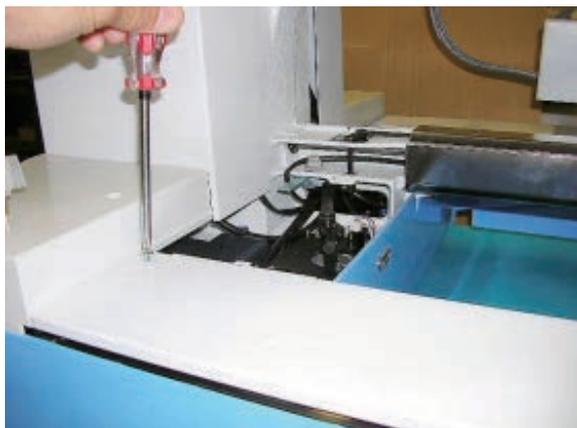
2. Loosen lock nut for tension adjustment screw.
