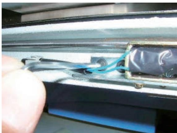
5. Exchange keeper solenoid. (Fixing screw 2 pcs)
