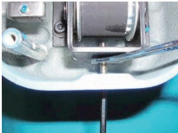
3. Loosen tension screw so as to move tension.
