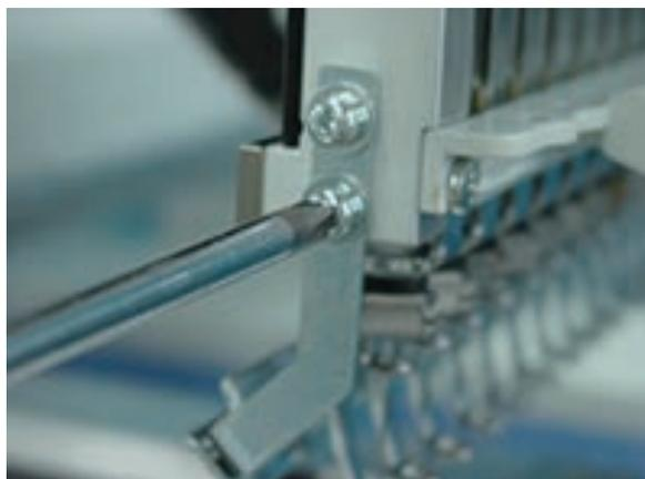
2. Please put out and withdraw thread catcher by your finger and fix holder position at smoothly moving position.
