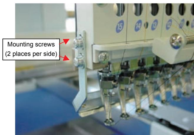
2. Fix stud bolts to the position where the screws are removed at the step 1.
