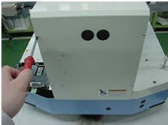
2. Remove pointer. (Fixing screw 1 pcs)
