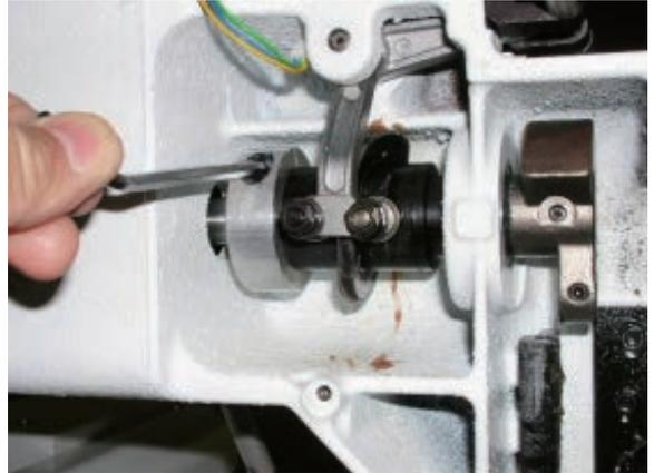
14. Loosen the screw on upper shaft collar.
