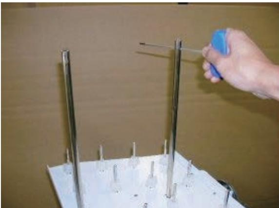
4. Remove 8 fixing screws and thread stand.
