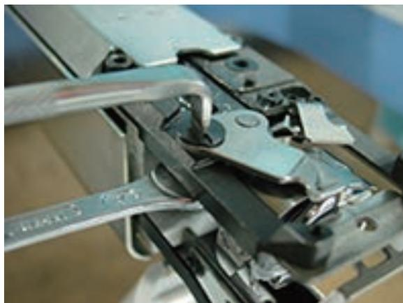
7. Referring to [3-6-4 Adjustment of moving knife and fixed knife], check how well thread is cut and adjust, then finish this process.
