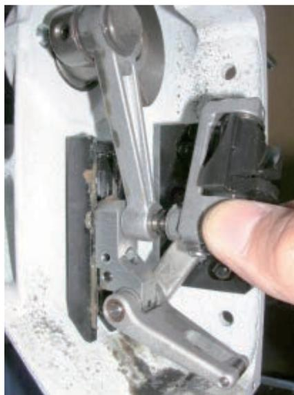
9. Remove rod ass'y. (Fixing screw 2 pcs)
