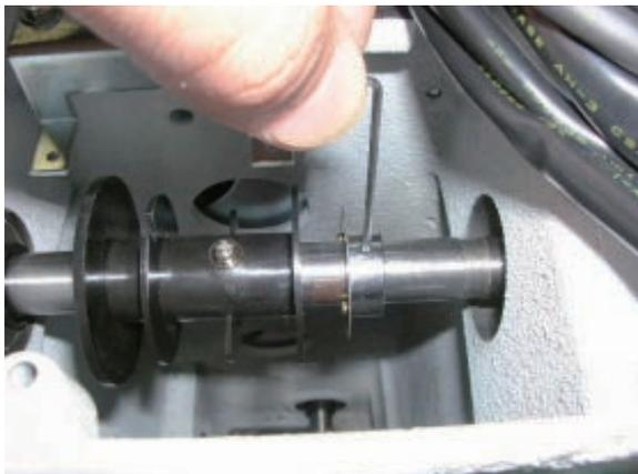
19. Loosen the screw on upper shaft collar.
