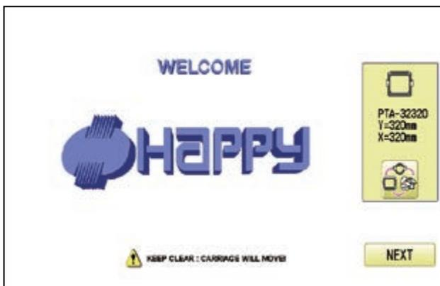
2. Press **NEXT** while pressing **START/STOP** button at the screen of the control box after booting the machine.
