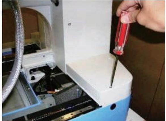
5. Remove the cover H. (Fixing screw 6 pcs)
