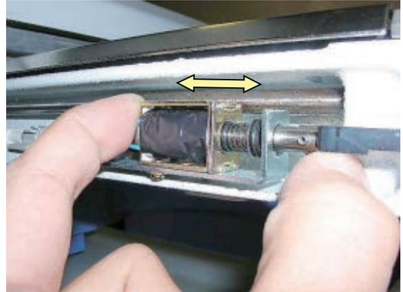
3. Insert keeper positioning gauge (Bobbin) into rotary hook.
