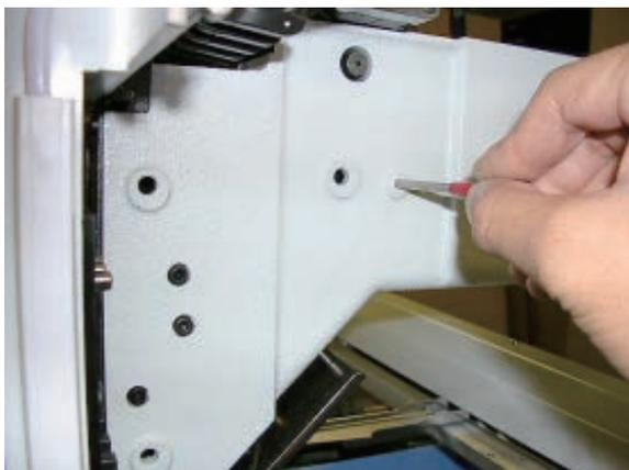
4. Turn take up lever barrel cam slowly and insert positioning pin into pin groove.
