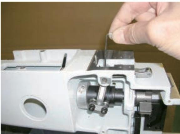
12. Pull out Take-up lever drive shaft and take off the crank ass'y.
