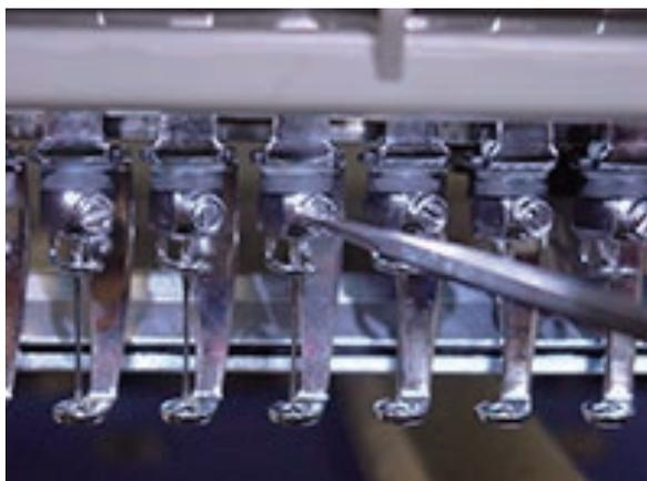
3. Remove pressure foot. (Fixing screw 1 pcs)
