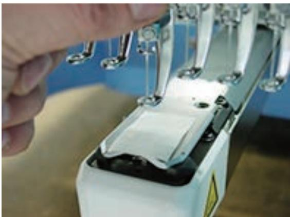
5. Reverse-rotate an upper axis, raise a needle bar, and unite with C [270 degrees].
