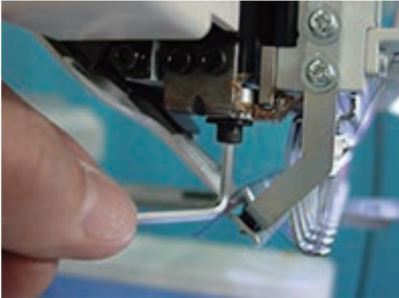
2. After adjustment, check and adjust needle drop to finish
