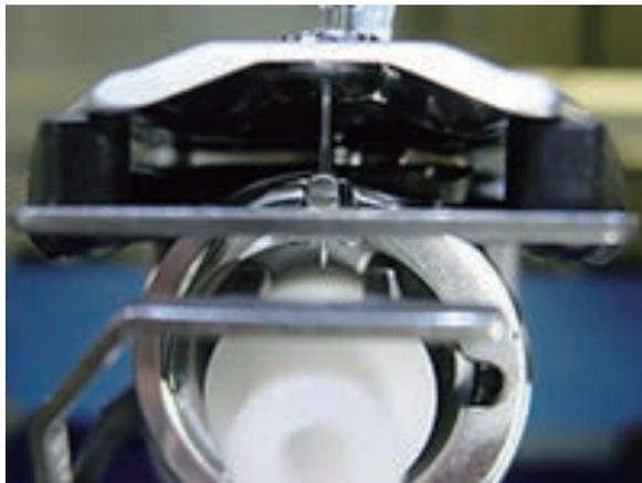
9. Tighten the screw of needle bar boss.
