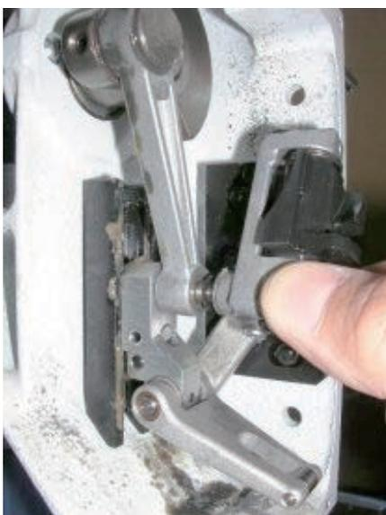
2. Remove "Screw on crank pin" and take off "Rod ass'y".
