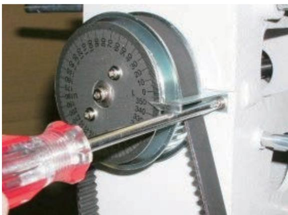
3. Loosen the screw on tension shaft ass'y.
