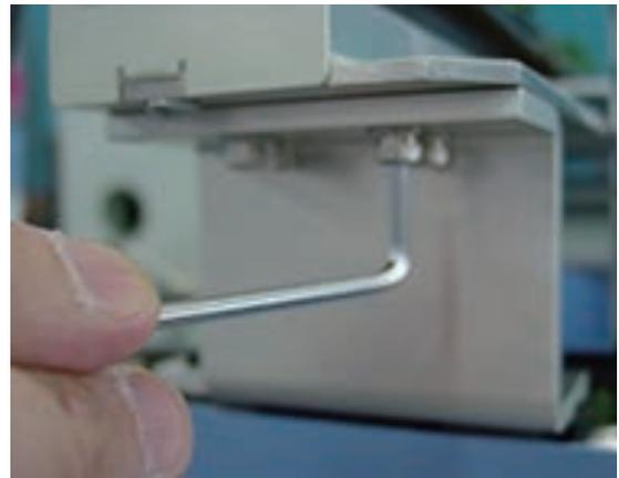
14. Check no gap between pin and carriage then fix screw of drive pulley.
