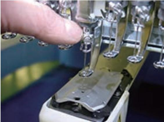
2. Turn upper shaft and set needle near to the lowest needle position [L] to adjust positioning plate ass'y.
