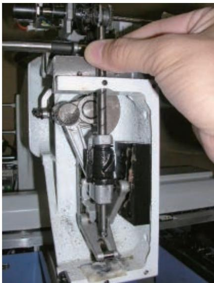
8. Remove needle bar driver ass'y.
