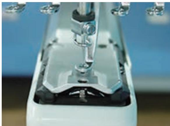
3. Adjust position of unit assembly so that needle comes to center against needle hole on needle plate and fix screws.
