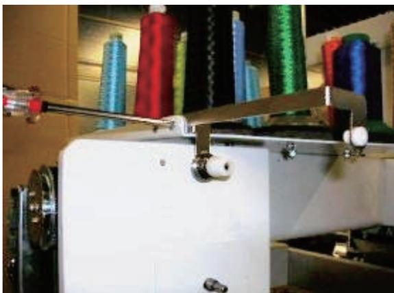
9. Remove the cover B. (Fixing screw 2 pcs)
