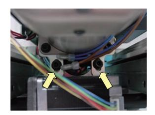
4. Adjust motor belt tension.
