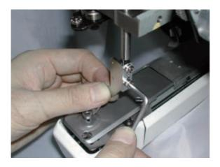
2. Loosen the screw which fixes guide bar boss.
