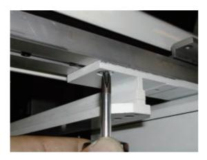
6. Loosen screw for tension.
