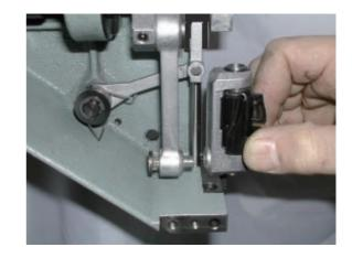
3. Loosen screw on rod pin to remove rod.
