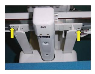
10. Remove the thread tension ass'y.
