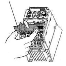
3. Install inverter in the machine with two screws tightened.
