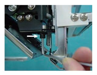
After adjustment, check and adjust needle drop to finish Please refer to [3-3-4 Adjustment of needle position (back and forth)].
