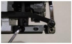
2. Insert keeper positioning gauge (Bobbin) into rotary hook.
