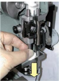
4. Loosen screw on lower part of needle bar driver ass'y.
