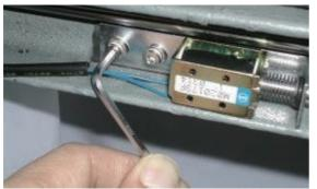
Loosen screw on stopper bracket.
