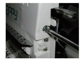
2. Disconnect TC cable and limit switch cable.
