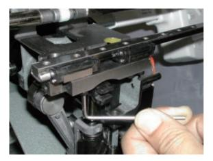
After remove pressure foot spring 2, remove pressure foot guide bar to up side.
