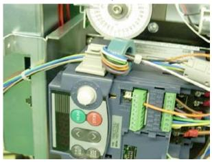
7. Remove two screws shown in the following figure and inverter.
