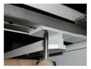
Loosen fixing screw for tension pulley bracket slightly. (front side)
