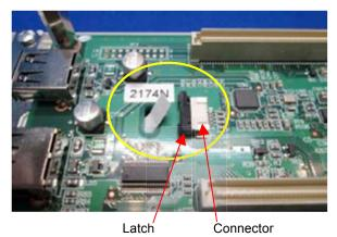
When you pull the latch to cord side, the cord release. When you push the latch to connector side, the cord fixed.
