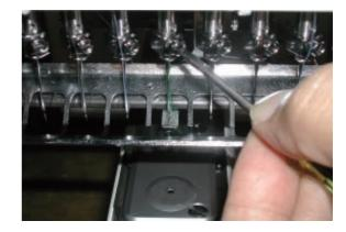
7. Loosen needle bar boss and needle bar boss B.
