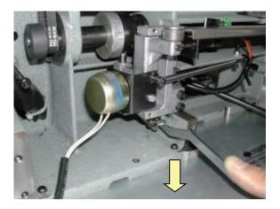
Insert 0.2mm thickness gauge between cam and roller and adjust the clearance [0.2mm] between cam and roller by adjusting screw.)
