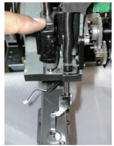
Adjust the center between needle hole of needle plate and hole of pressure foot.
