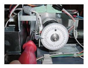
Loosen screws on upper shaft collar, upper pulley and drive pulley.
