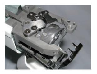
If necessary, please refer to [3-6-8 Adjustment of moving knife and fixed knife] and check how well thread is cut, then finish. 1.Remove Needle plate and Cover (front).
