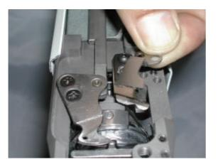
4. Tighten fixed knife pushing to forward as full as possible.
