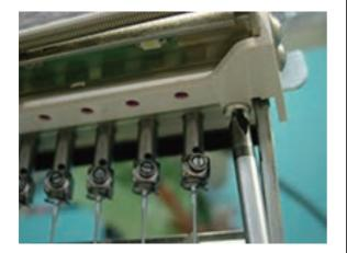
4. Remove thread adjusting spring and spring holder.
