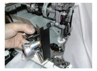
2. Referring to [3-2-4 Exchange of needle bar driver], remove needle bar driver ass'y.
