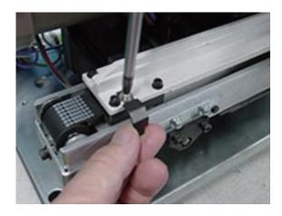
6. Check of interference between detecting plate and sensor
