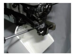
3. Remove keeper solenoid ass'y.
