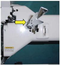
18. Remove cover (light). (Remove screw in arrow mark)
