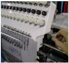
5. Put in SIMM [0.05mm] between a moving head and LM guide.
