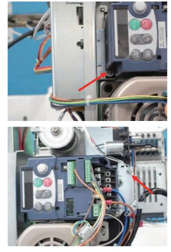
4. Tighten screws with screwdriver to install power cable and motor cable per the following connection diagram.
