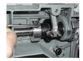
5. Loosen screw on crank.
