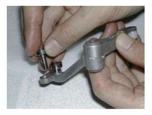
Insert bering positioning gauge [4.85mm] between bering and bering , and then tighten roller shaft ass'y.
