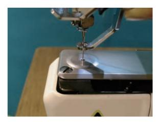
4. After adjustment, please be sure to check and adjust clearance between needle and shuttle hook. Please refer to [3-5-1 Adjustment of rotary hook timing].
