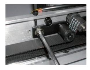
10. Tighten fixing screw for tension pulley bracket. (rear side)
