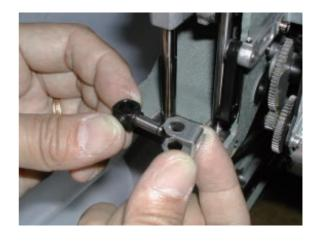
6.Assemble the pressure foot gude bar and pressure foot.
