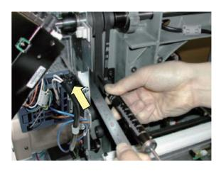
Gauge in the near center between drive pulley and motor pulley.
