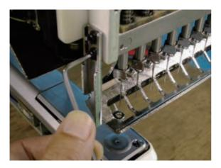
Hold down the pressurefoot and take the hook in and out by finger to check movement of hook goes smoothly. Check this at 1th , 6<sup>th</sup> , 12<sup>th</sup> needle.
