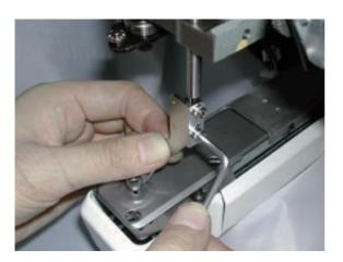
Adjust the height of pressure foot guide bar to finish.
