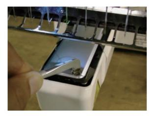
Pull bobbin thread toward arrow mark and see that bobbin thread comes off with tensile gauge [20-25g].
