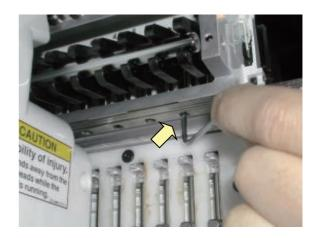
Turn the drive shaft B screw for manual operation, and make it the 12th needles.
