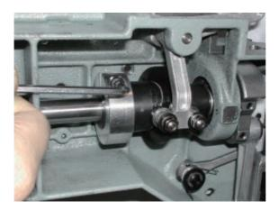
14. Remove bearing retainer.
