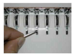
2. Move adjuster position up and down with small frat-head driver to change stroke.
