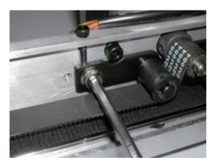
8. Loosen screw (rear) slightly to the extent that tensionbracket moves.
