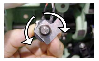
Turning the shaft too much make \* disappear, and turn the shaft back and forth, and adjust the position so that continuous beep is made.  Install potentiometer at the 6<sup>th</sup> position while beep is made and fix it with setscrew.
