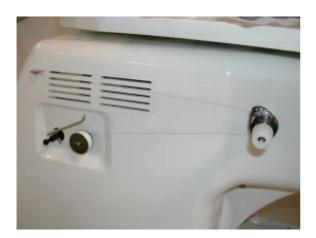
8. Adjust the inclination of Winder bracket ass'y in accordance with thread winding condition.
