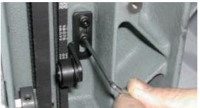
3. Loosen screws on upper shaft collar,
