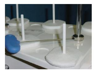
7. Remove thread guide pillar and thread stand.
