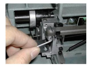
8. Remove thread cutting driver ass'y .
