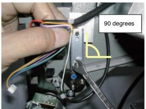
Adjust the height of pressure foot guide bar.
