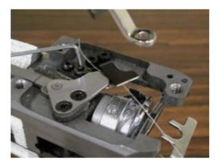
5. Tighten lock nut. (Don't move adjusting screw.)
