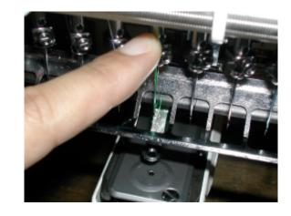
4. Adjust position of unit assembly so that needle comes to center against needle hole on needle plate.
