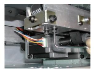
7. Adjust belt tension, to use belt tension gauge.
