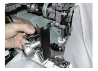
2. Loosen screw on main shaft in head.
