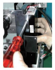
4. Loosen screw on fasten collar for take-up lever cam.
