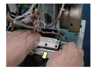
5. Assemble detecting plate.
