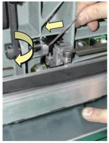
5. Tighten screw on thread cut cam when moving knife began to open.
