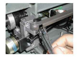
On checking the clearance [0.2mm] between cam and roller by using <u>0.2mm thikness gauge</u>.
