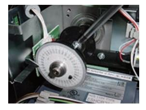
2. Turn upper shaft so that needle bar driver ass'y comes in the bottom.
