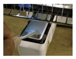
2. Remove knife drive shaft retainer.
