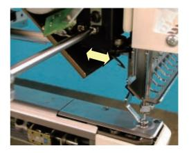
\* Insert Lower rail to between the two bearing deeply. (This is for setting of Moving head completely.)
