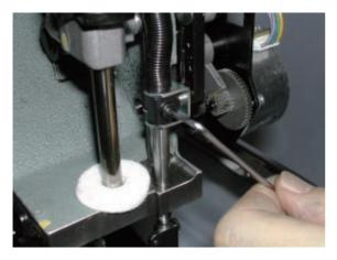
3. Rotate the upper shaft to be lowest point [0 degrees].
