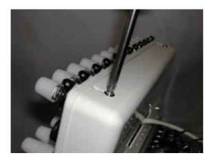
4. Remove thread tension bracket.
