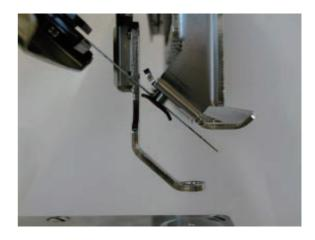
3. Insert positioning gauge [47.5±0.1mm] between lower part of moving head and holder (upper) and mount it vertical.
