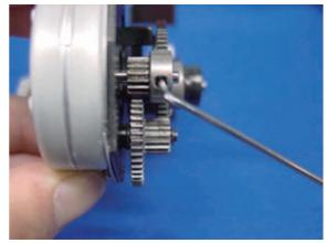
7. Adjust position of pulse motor then fix it.
