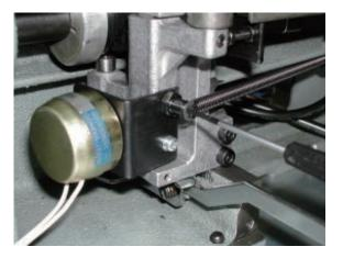
7. Remove drive link ass'y from thread cutting driver ass'y .
