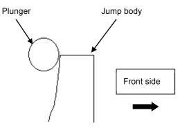
7. Adjust upper shaft to be [180 degrees] and tip of the body has to be same as the picture below.
