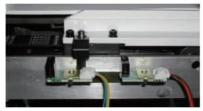
Loosen the screw for coupling of the Y carriage.
