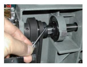
4. Loosen screw on fasten collar for take-up lever cam.
