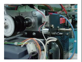
2. Assemble the left cover with keeping the space between shaft and the cover hole.
