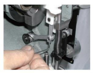
4. If you remove the pressure foot link B ass'y, first remove the pressure foot cam collar and pressure foot drive cam.
