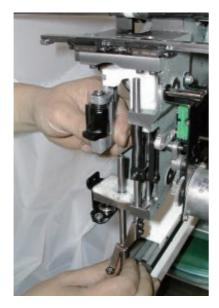
2. Loosen the screw which fixes guide shaft then move the guide shaft lower.
