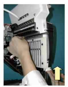
6. Tighten an inside screw (arrow portion in a figure).
