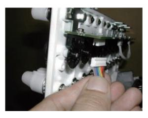
3. Remove front cover on front panel.
