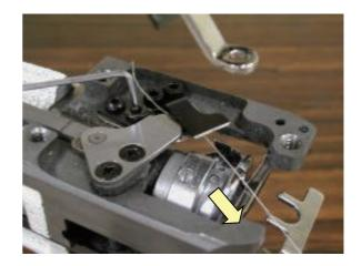
2. Close moving knife like putting bobbin thread between moving knife and bobbin thread holder.
