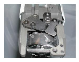
7. On Checking that the knife began to open, at [116 degrees(+0 / -2degrees)] work has finished.
