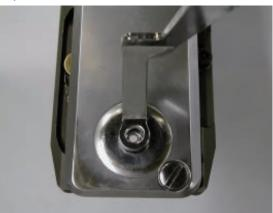
Insert thickness gauge [1.2mm] between needle plate and pressure foot then tighten the screw which fixes guide bar block.
