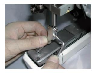
10. Assemble sensor board ass'y.
