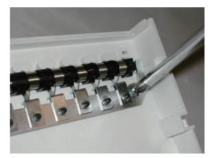
5. Exchange thread adjusting spring.
