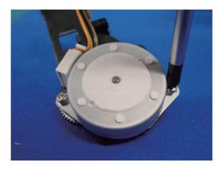
6. Assemble the drive gear A.
