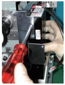
2. Loosen screw on thread cut cam.
