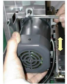
5. Tighten screw on motor bracket.
