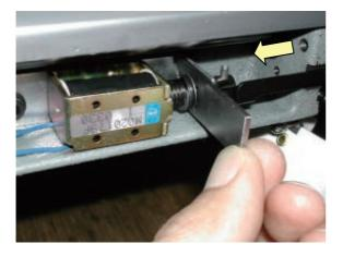
Adjust solenoid base where tip of keeper contacts slightly to the gauge then tighten bracket screw.
