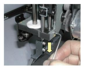
3. If you exchange block ass'y, loosen the screw which fixes pressure foot link A then remove block ass'y.
