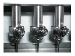
10. Tighten the screw of needle bar boss.
