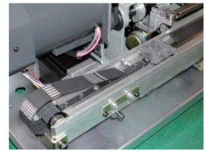
10. Set belt to belt groove of guide frame base.
