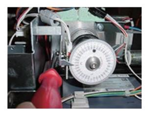
9. Remove bobbin winder and power supply.
