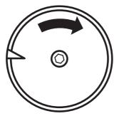
4. Turn thread cut cam clock-wise while pushing release lever down.
