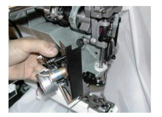
Referring to [3-2-4 Exchange of needle bar driver], remove needle bar driver ass'y.
