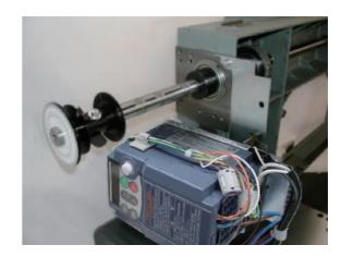
7. Remove upper pulley and timing belt. Install good timing belt.
