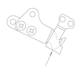
Adjustment of clearance between moving knife and fixed knife is where both tip of then are attached.
