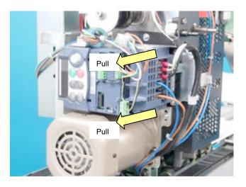
4. Loosen screw with Phillips screwdriver for precision instrument and remove 9 cables. (Cable color: ORANGE, BROWN, PURPLE, WHITE, GREEN, BLUE, YELLOW, BLACK, and GLAY)
