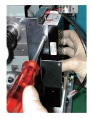
2. Remove timing detecting board ass'y.
