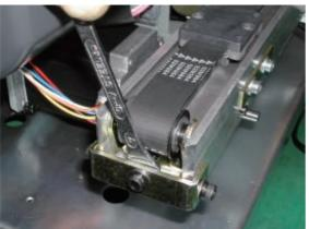
6. Loosen tension screw so as to move tension.
