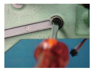
9. Assemble pressure foot guide bar and pressure foot.
