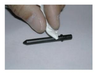
3. Put the designated grease on plunger part. <Grease> Shell Grease7 MIL-G-23827B
