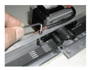
7. Remove the screw which fixes tension bracket.
