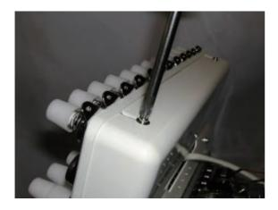
4. Remove thread tension bracket.
