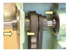
(3)Position of upper pulley is [2mm] from upper shaft collar.(3)Position of upper pulley is space from upper
