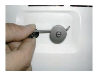
If the guide touches the bobbin adjust position of the winder bracket ass'y.
