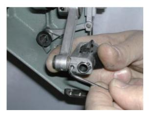
5. Remove needle bar driver ass'y.
