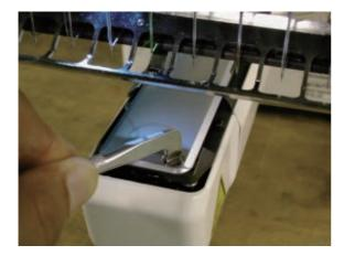
3. Tighten screw on rotary hook. (3 places)
