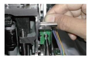
11. Adjust position of pressure foot guide plate A ass'y.
