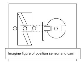
2. Set position where sensor on sensor board and slit don't cross to area where moving head doesn't move
