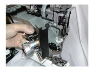
15. Install parts in reverse order to finish.For adjustment of fixing of each unit, please refer to process to adjust fixing of each unit.
