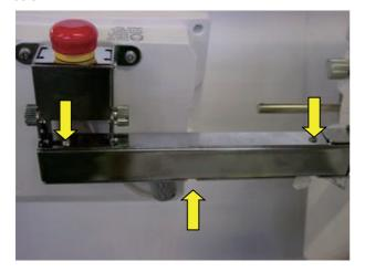
2. Disconnect the connectors indicated by the arrows in the figure below. Remove the screw that fixes cables.
