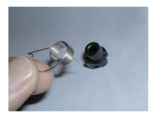
3. Remove thread adjusting spring ass'y.
