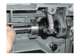
5. Loosen screw on crank.
