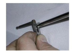
Setting drive link hole to moving knife, insert knife drive shaft assembly.
