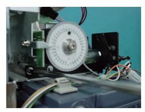
6. Adjust bobbin thread tension [30g] by tension gauge.
