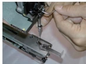
Before terminates the adjustment, reconfirm procedure 5, Needle hole of needle plate and hole of pressure foot to be centered.
