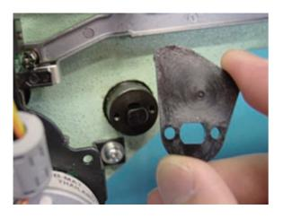
3. Put on grease to pressure foot cam.
