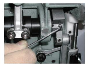
Pull out upper shaft (to the extent that shaft comes off from take-up lever cam).
