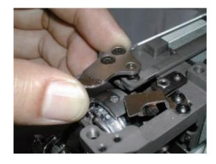
6. Pushing down moving knife and knife drive shaft retainer like putting them together, fix knife drive shaft retainer.# Fix so that there is no backlash in upward and downward direction and to to move lightly.
