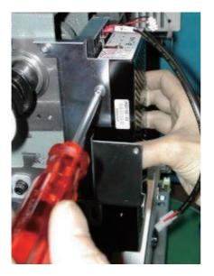
2. Adjust tension of timing belt.
