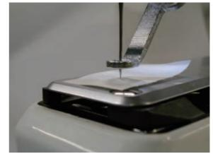
Reverse-rotate an upper axis, raise a needle bar, and unite with C [275 degrees].
