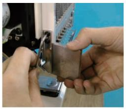
5. Thread catcher device should be adjusted if above clearance is not keepable.
