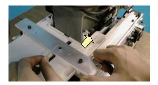
3. Hold the left side of arm to body and tighten screw.
