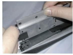
Do not put belt tooth on the innermost groove of the connecting plate.
