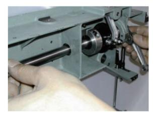
11. Loosen collar screw on take-up lever cam.
