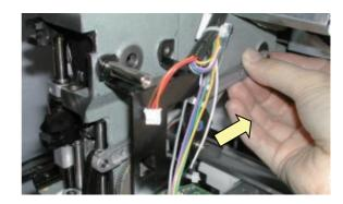
6. Put on grease to bady and oil bush of pressure foot lever
