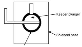
Clearance between keeper plunger and solenoid base should be kept as much as equally.
