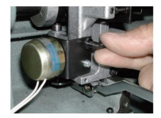
14. Fix Y carriage bracket (left) to the machine.Fix the base with state of pushing it down.Tighten drive shaft with screw.
