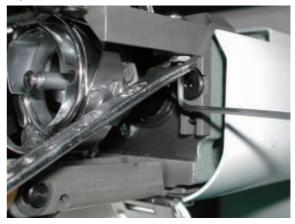
4. Cut thread and check how well it is cut. Use two polyester threads for checking.
