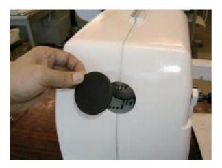
13. Remove cover (left). (Remove screw in arrow mark)
