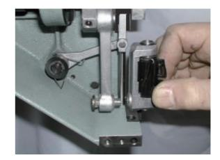
8.Remove circuit board assembly for timing detecting board.
