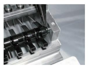
8. Remove the take up lever shaft first then remove the takeup lever.
