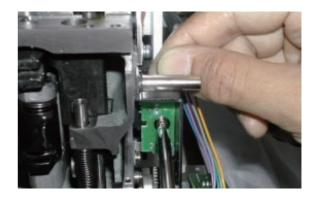
3.Remove pressure foot and pressure foot guide bar.
