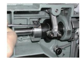
5. Loosen screw on crank.
