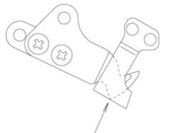
Adjustment of clearance between moving knife and fixed knife is where both tip of then are attached.
