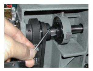
12. Loosen screw on crank.
