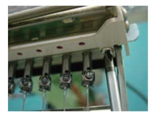
2. Loosen screw to the extent that thread holder moves.
