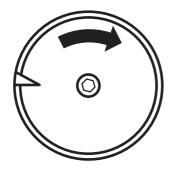
Move circuit board up and down and set to position where LED 2 disappears at [0 degree], then fix with screw.
