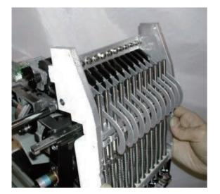
2. Exchange of needle bar boss guide plate.
