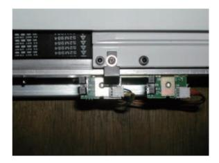
Adjust by bending detecting plate by hand if you find any interference with sensor or connector.
