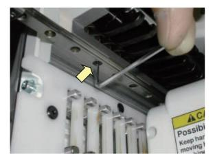
11. Check center (right and left)(back and forth) of needle and needle hole of needle plate.(Needle No.1 ,6 and 12.)
