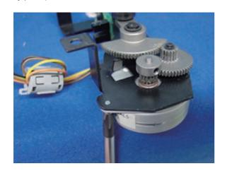
8. Continue to conduct [Adjust the pressure foot bracket ass'y].
