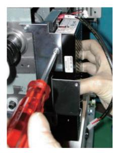
10. Loosen screw on upper shaft collar, upper pulley, drive pulley.
