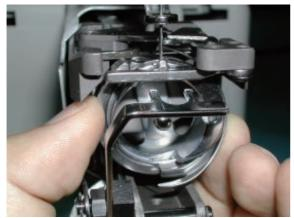
At this moment, clearance between needle and rotary hook should be [0.1-0.2mm].
