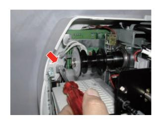
17. Remove an arrow marked screw which fixes hold arm D.
