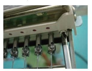
Block has spring groove to be able to adjust in three steps
