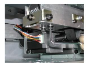
9. Tighten lock nut for tension adjustment screw.
