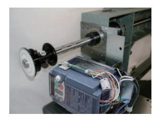
7. Remove drive pulley and motor belt. Install good motor belt.
