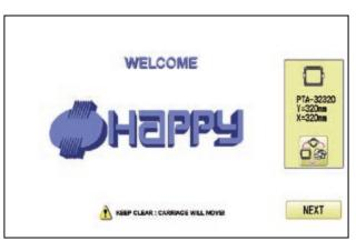
3. Press NEXT while pressing START/STOP button at the screen of the control box after booting the machine.
