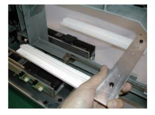
2. Hold arm to backward and tighten only hithermost screw.
