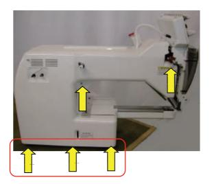
When the cover is fixed by 3 screws as above picture, please remove these screws.
