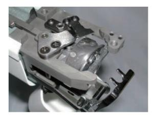
6. With release lever being pushed down, turn upper shaft
