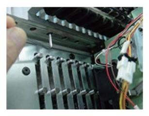
3. Remove front cover on front panel.
