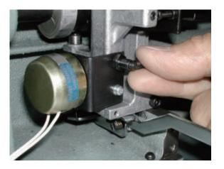
9. Remove thread cutting roller.
