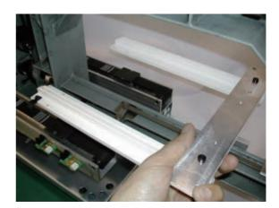
3. Loosen the screw for coupling of the Y carriage.
