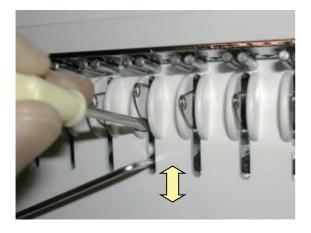
3. After adjustment, tighten screw to finish.
