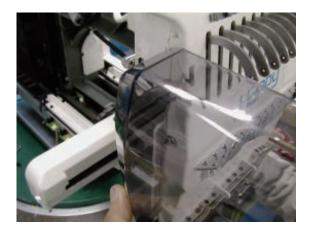
4. Referring to [3-3-3 Assemble the moving head], remove moving head.
