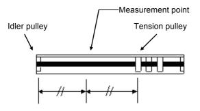
Adjustment, tighten fixing screw for tension pulley bracket.
