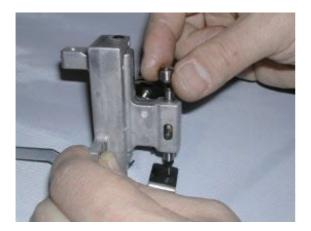
11. Fix thread cutting driver ass'y to the machine.
