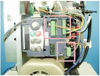
Remove screws with Phillips screwdriver and remove power cable and motor cable. (Cable color: GLAY, WHITE BLACK, BLUE, and BROWN)
