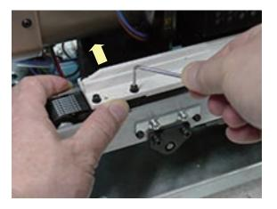
4. Hold the right side of arm to arrow pointed direction at below picture and tighten screw.
