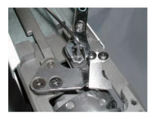
3. Adjust height of bobbin thread holder with adjusting screw.
