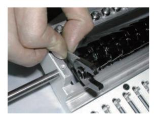
9. Install good take-up lever assembly with plastic washer, E-ring.
