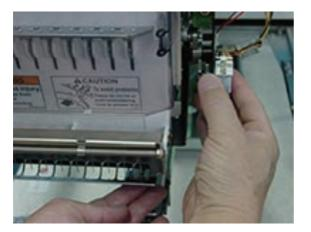
4. Adjust position of pressure foot guide plate B ass'y.
