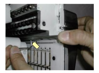
At this time, a moving head is pushed from the front and it is LM guide.
