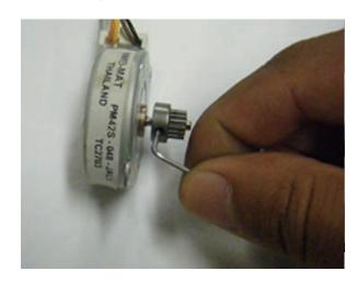
Install Drive gear on good Pulse motor
