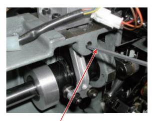
Push take-up lever drive shaft by slender shaft. (Hexagon wrench etc.)
