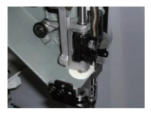
3. When dial disc reads [0 degree], fix detecting disk.
