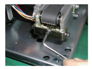
8. Tighten screw on tension.
