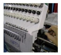
9. Tighten an inside screw (arrow portion in a figure).
