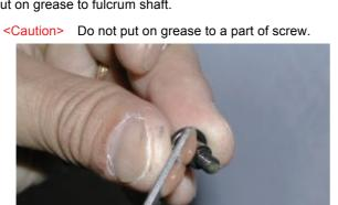
8. Assemble pressure foot drive lever ass'y.
