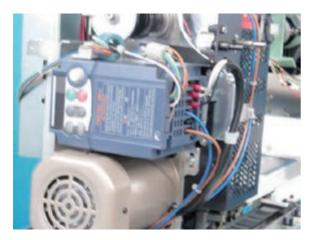
3. Loosen screw on motor bracket.
