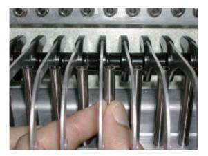
9. While pressing needle bar spring, insert good needle bar.
