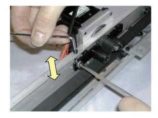
9. Tighten fixing screw for tension pulley bracket. (front side)
