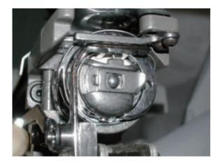
3. Insert [2.0mm] clearance gauge between solenoid base and slider then pull in keeper solenoid and keeper rod.
