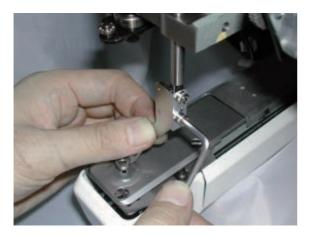
5.Exchange pressure foot drive lever ass'y.
