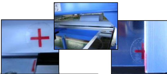
Center mark position of X axis Center mark position of Y axis
